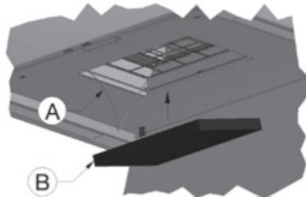
Compress spring (A) and turn it downwards and place monoblock filter (B) into the cooker hood.
