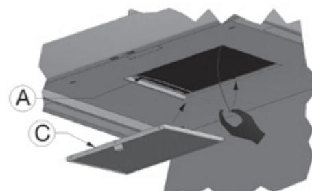
Close lock spring (A) by compressing it again and securing it in the slot provided. Place grease filter (C) in the cooker hood again.
