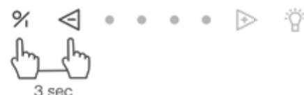
The function can be switched on by pressing the ① and ③ keys at the same time for 3 seconds.
